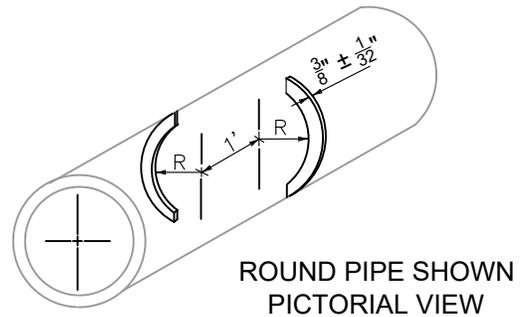
CURVE CUTS ARE ACCEPTABLE PROVIDED THE CONTROL DIMENSION IS MAINTAINED (TYPICAL FOR ELLIPTICAL AND ROUND PIPE)
