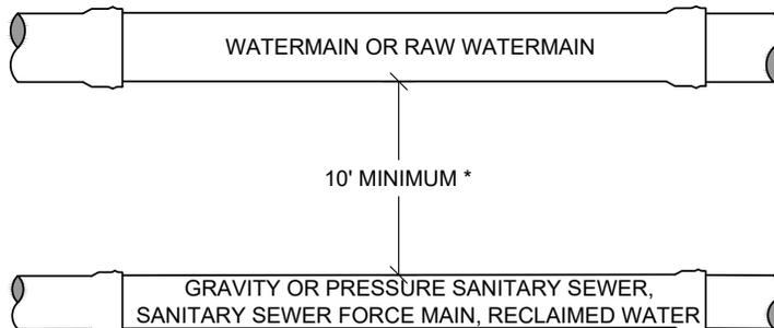
\* 3' FOR GRAVITY SEWER WHERE THE BOTTOM OF THE WATERMAIN IS LAID AT LEAST 6" ABOVE THE TOP OF THE GRAVITY SEWER.
