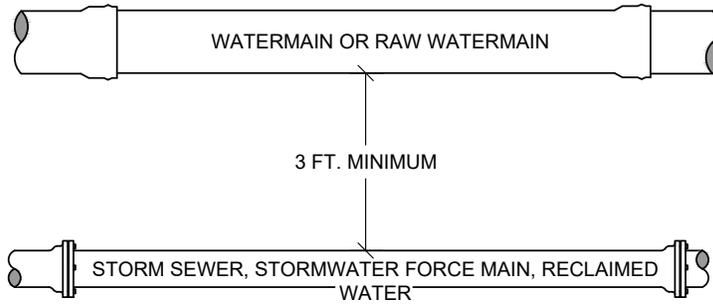
NOTE: CASE # 1 SHALL BE USED FOR ALL UNDERGROUND ELECTRICAL UTILITIES, TELECOMMUNICATION UTILITIES, GAS UTILITIES AND OTHER CONDUITS, CABLE, WIRE ETC.
