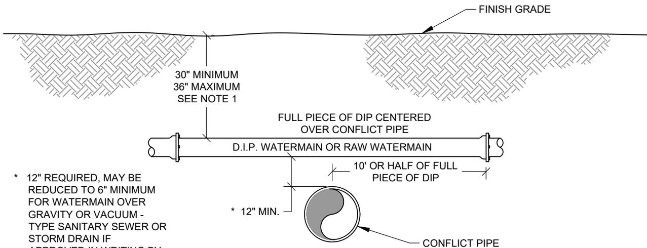
\* 12" REQUIRED, MAY BE REDUCED TO 6" MINIMUM FOR WATERMAIN OVER GRAVITY OR VACUUM - TYPE SANITARY SEWER OR STORM DRAIN IF APPROVED IN WRITING BY THE TOWN OF JUPITER.
